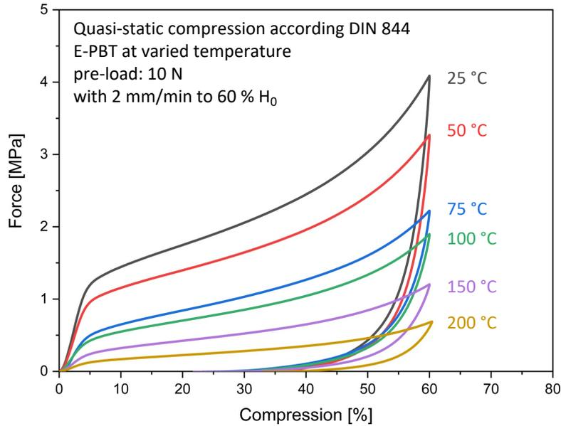
**FIGURE 2:** Results of compression tests carried out on E-PBT ( $229 \text{ kg/m}^3$ ) at different temperatures.
