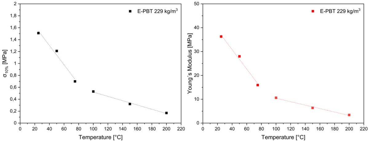
**FIGURE 3:** Temperature dependency of the stress at strain (10%) and the Young's modulus of E-PBT taken from the compression tests.
