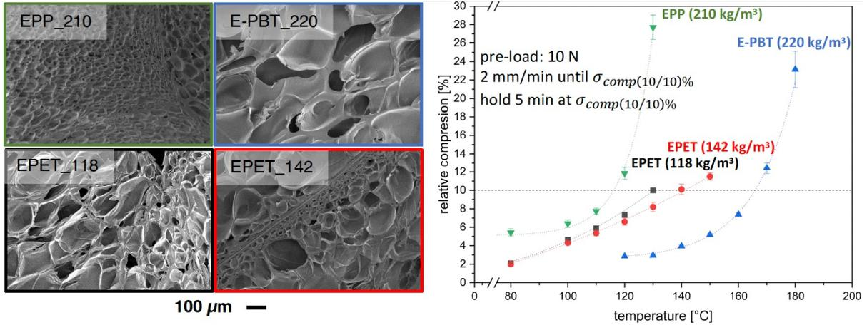
**FIGURE 4:** Left: SEM images of the investigated foam structures. Right: Relative compression during the creep test at different temperature steps
