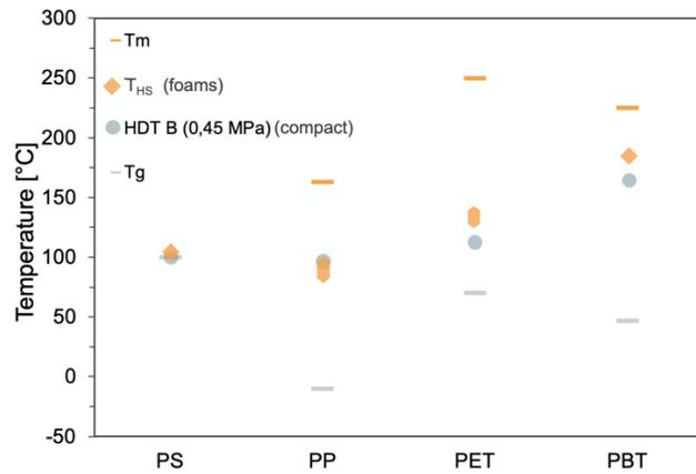
**FIGURE 5:** Thermal data ( $T_g$  and  $T_m$ ) as well as heat deflection temperature (HDT/0.45 MPa) extracted from data sheets as well as the  $T_{HS}$  measured with the described approach (data partially taken from Himmelsbach et al. [10]).
