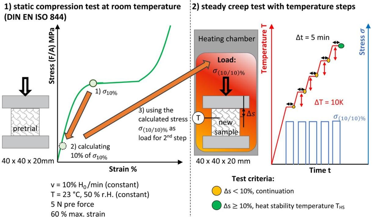
**FIGURE 1:** Scheme of the measurement principle. In a first step (left) compression test according to DIN EN ISO 844 are carried out to determine a very low load ( $\sigma_{(10/10)\%}$ ), which is applied in the second step (right) – a creep test with temperature steps. (image by Himmelsbach et al. [10], used under CC BY 4.0)
