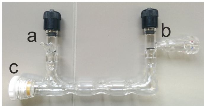
Figure S3. Rubidium presaturation cell. a) Valve and gas inflow. b) Valve for gas outflow. Via the flange a connection to the optical pumping cell is realized. c) Rubidium filling port with PTFE gasket screw. The indentations at the bottom of the cell serve as reservoirs for the Rb. They avoid the Rb to flow and accumulate in the right part of the cell and define the surface area of the Rb, which is exposed to the gas flow. For measurement “series II” the bottom of all four bulges were filled with Rb, while in “series I” only the first two bulges were filled.
