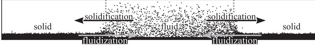
Figure 5.5: Sketch of the particle fluxes across the phase boundary for pure vertical forcing. The background image is taken from Fig. 5.1b.
