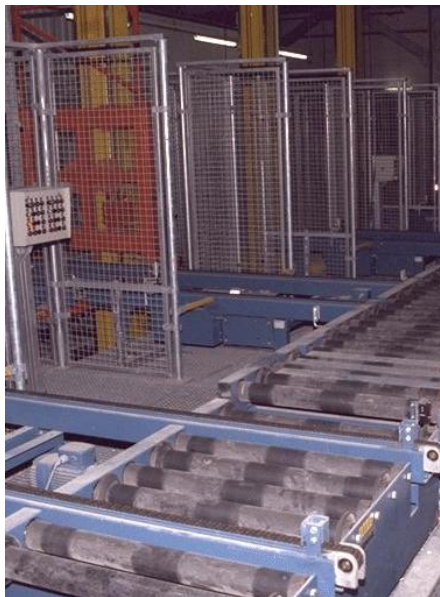
Fig. 1 Pallet elevators at the distribution center of Herlitz with a single waiting slot in front of each
