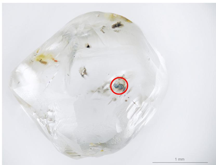
**Figure 7.1.** Diamond containing ferropericlase inclusion AZ2 (indicated with a red circle).
