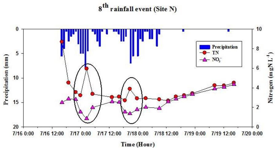
Figure 2.11 Variations of TN and nitrate concentrations at Site N during 8<sup>th</sup> rain event
