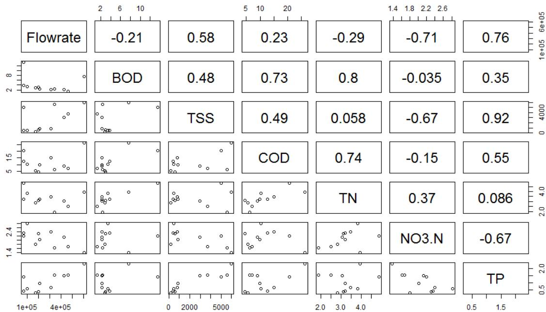
Figure 2.10 Scatter plots and correlation coefficients among water quality parameters at Site N during rain events for 2 years (2009–2010)
