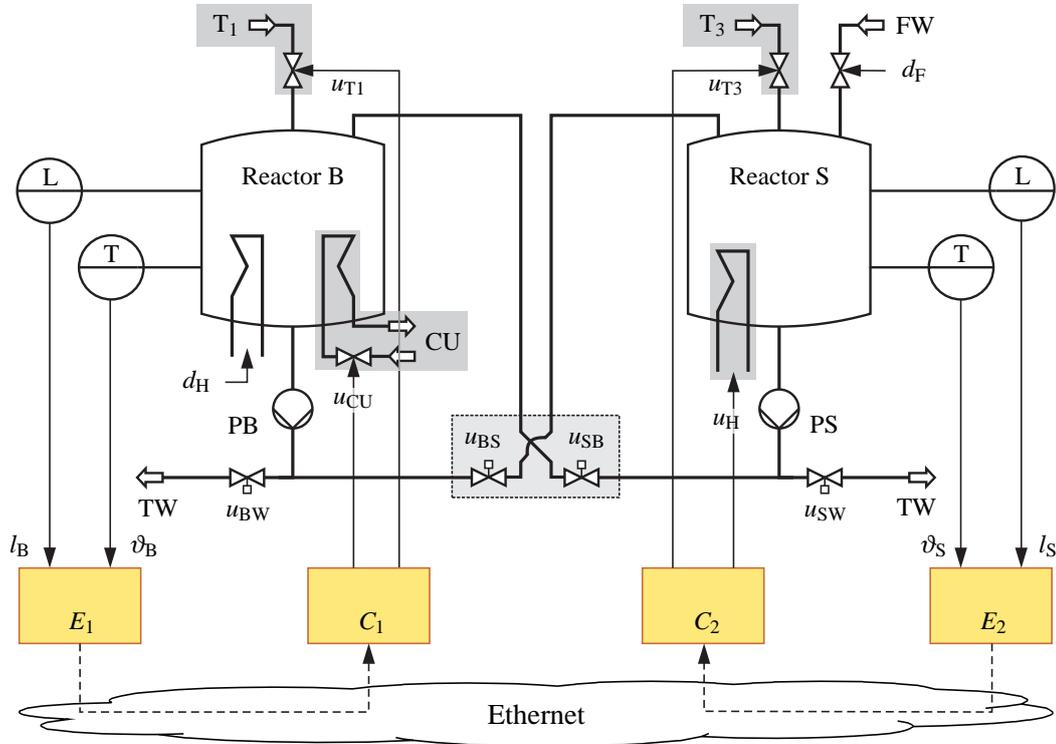
Figure 12.2: Experimental setup of the continuous flow process
