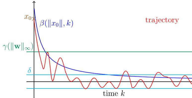
Figure 2.1: Input-to-State practical Stability for  $\Sigma$
