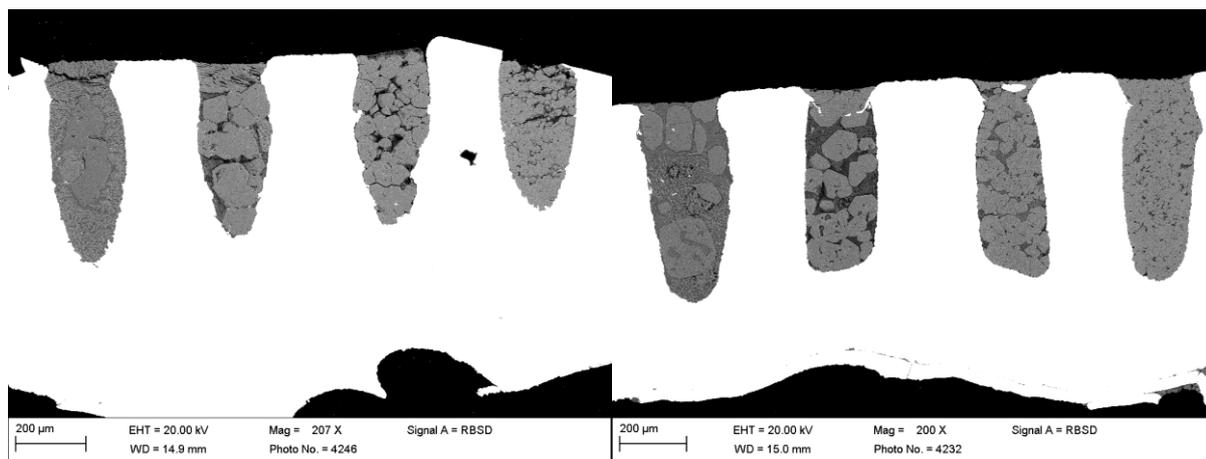
**Figure 3.2-2.** Backscattered electron image of two experiments performed at 6 GPa and 1500 °C (V706, left) and at 1300 °C (V707, right). From each experiment from left to right the sample chambers were refilled with A, B, C and D starting mixtures (see Table 3.2-1), therefore the water content increases from right to left.
