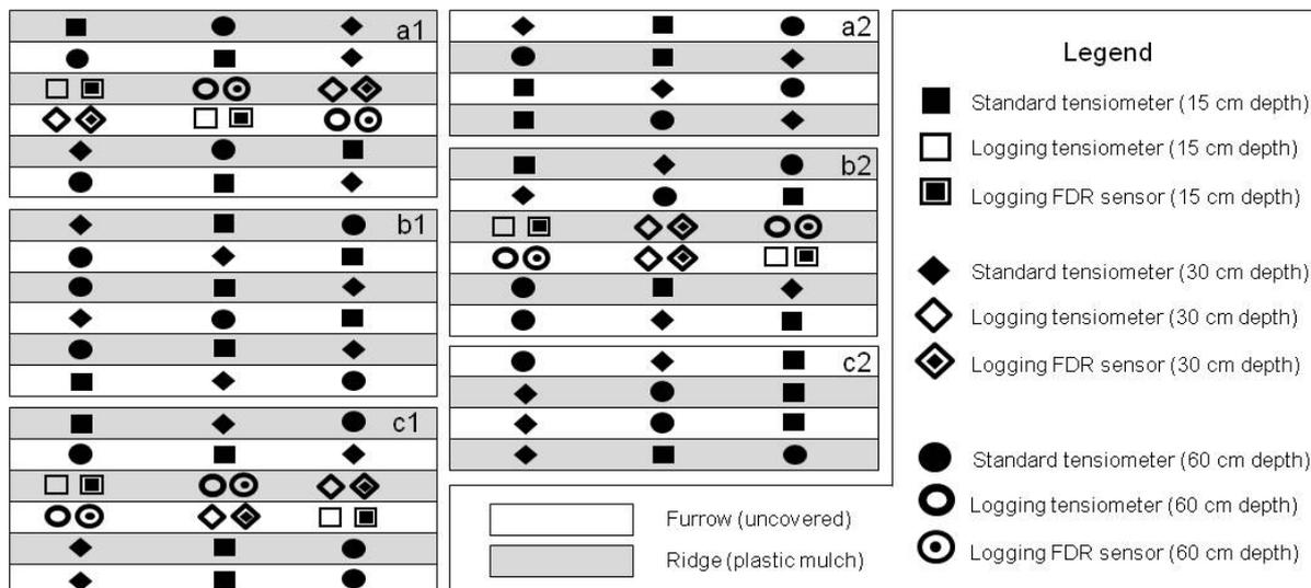
**Fig. 2.** Monitoring network of standard tensiometers, continuously recording tensiometers and FDR sensors; subplots a, b and c refers to different slope locations (a: upper slope, b: middle slope, c: lower slope), 1: field site 1 and 2: field site 2. The distance between subplots was approximately 15 and 30 m on field site 1 and 2, respectively.
