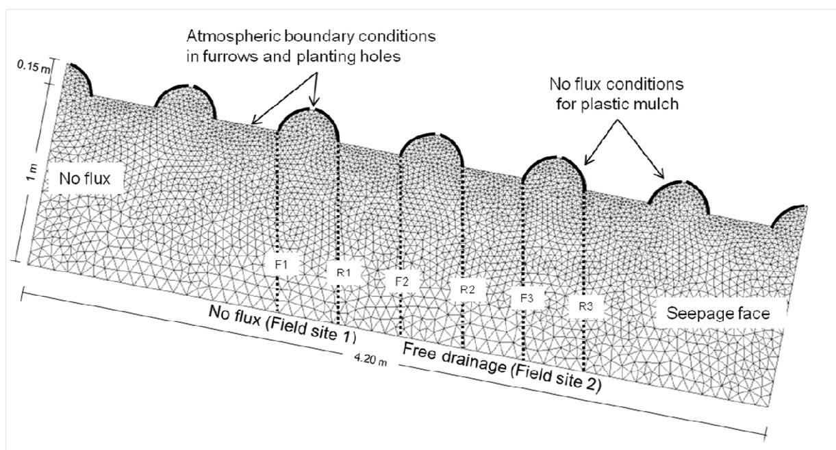
**Fig. 4.** Boundary conditions of the model simulations; note that the bottom boundary varies between the two field sites; vertical meshlines F1-3 and R1-3 were included to calculate lateral water fluxes (see Fig.9); for simulation of ridges without coverage (RT) and conventional tillage (CT) atmospheric boundary conditions were implemented at the entire surface.
