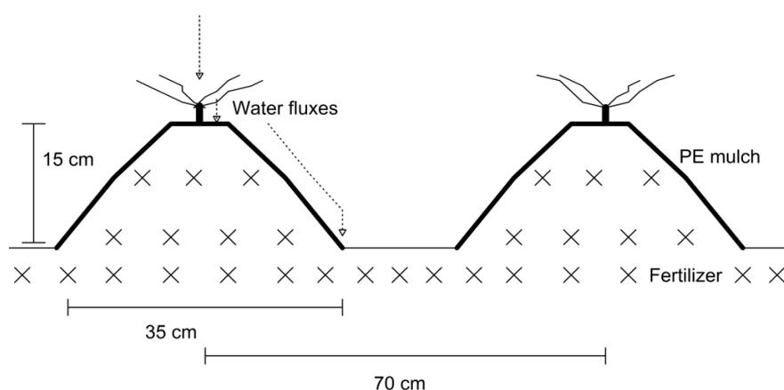
**Figure 1** Scheme of a typical ridge cultivation system with plastic mulching used for radish production in a temperate South Korean area with summer monsoonal climate. The water fluxes (  $\dashrightarrow$  ) and the distribution of fertilizer N (X) in the system are indicated.
