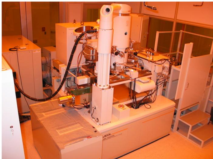
**Figure 3.5:** Image of Jeol JBX-9300FS<sup>2</sup>: This dedicated EBL tool is located in the clean room of the Cornell NanoScale Science and Technology Facility (CNF).
