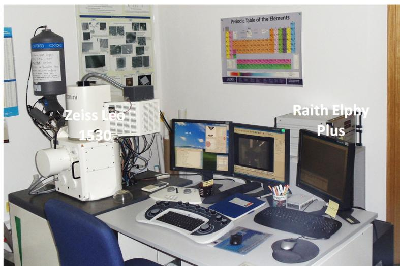
**Figure 3.1:** Image of the EBL facility in the Bayreuth Institute of Macromolecular Research: This tool consists of a Zeiss LEO 1530 equipped with a Raith Elphy Plus control unit.
