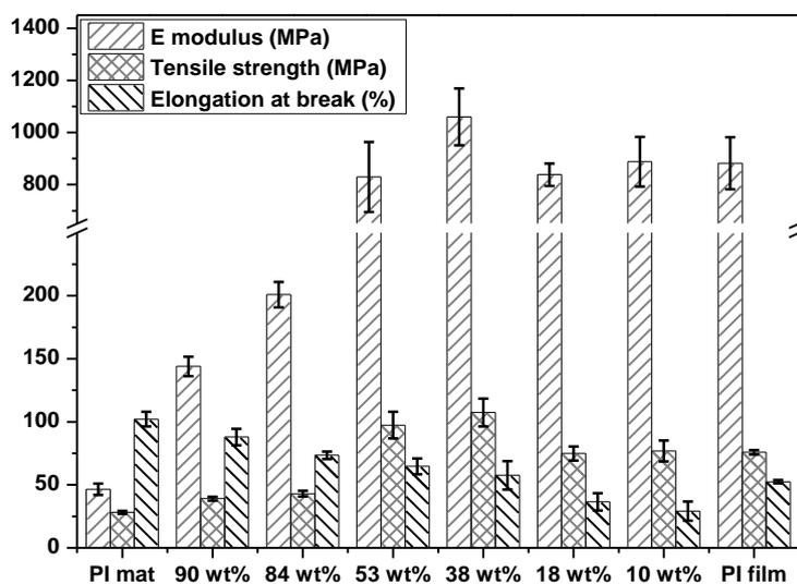
**Figure 6-S1** Bar chart of mechanical properties of self-reinforced PI nanofiber composites with as-electrospun PI nanofiber mats.
