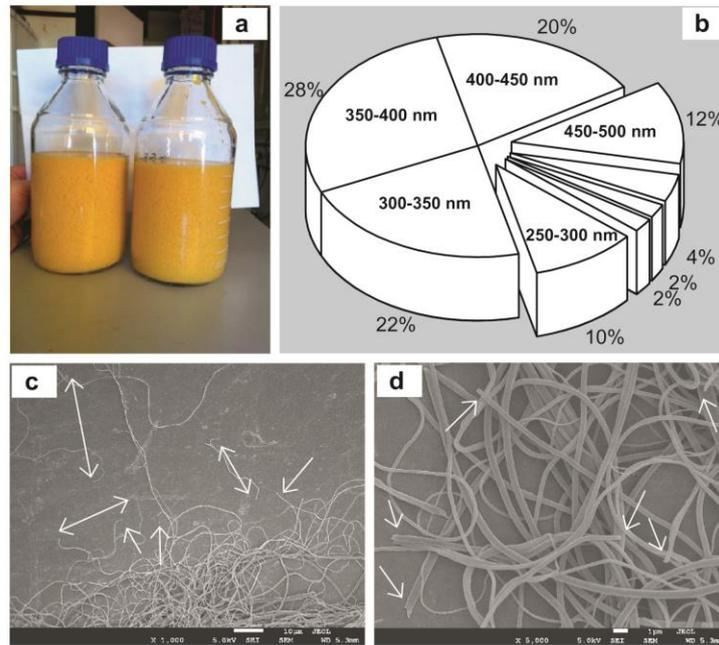
**Fig. 1.** Photograph of dispersions of electrospun fibers in isopropanol/water (30/70 w/w) after cutting (a), pie chart of the diameter distribution of PI nanofibers (b) and SEM micrograph of short PI nanofibers (c and d) with chain ends marked with white arrows. Scale bar of (c) = 10 μm and (d) = 1 μm.
