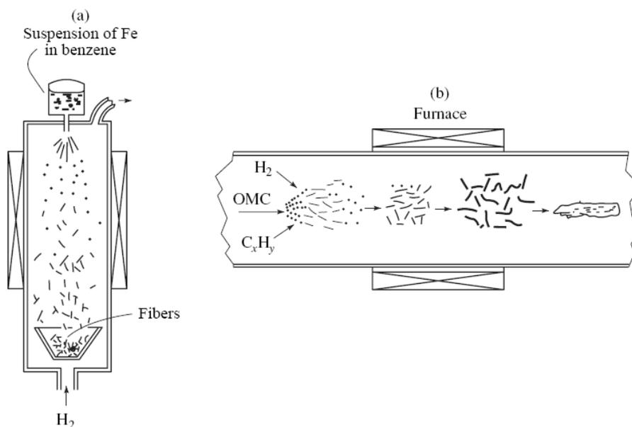
**Figure 1-9** Schemes of the growth of vapor grown carbon fibers in a gas flow: (a) a catalyst is introduced into the reactor as a suspension in a liquid hydrocarbon and (b) volatile organometallic compounds (OMC) are used[81].
