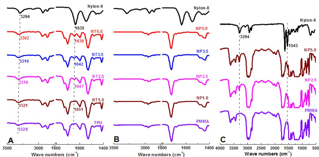
**Figure 2-10** (A and B) ATR-IR spectra of pure TPU film, pure PMMA film, nylon-6 nanofiber mat and short nylon-6 nanofiber reinforced TPU and PMMA composite films. (C) FT-IR spectra with transmission mode of pure PMMA film, nylon-6 nanofibers and composite films NP2.5 and NP5.0.
