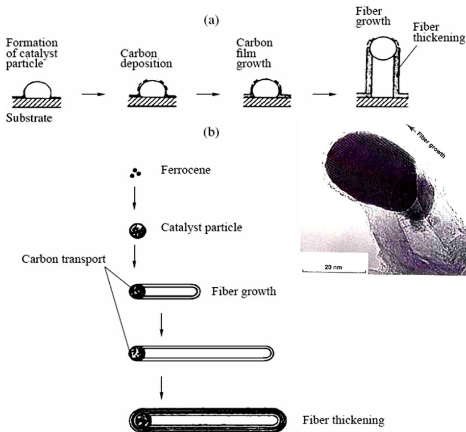
**Figure 1-10** Models of the growth of vapor grown carbon nanofibers, (a) on a substrate and (b) in a gas flow. Insert: seeded metallic particle at the end of the growing carbon nanofiber[81, 166].
