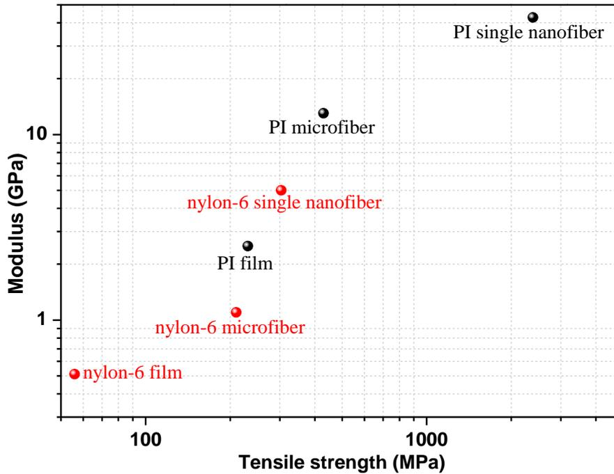
**Figure 1-17** Summary of mechanical properties of single nylon-6 and polyimide (PI) electrospun nanofibers compared with other formations (nanofiber mat, film, microfibrer, etc.). Nylon-6 film [5]; nylon-6 microfibrer [2]; nylon-6 single nanofiber [1, 3]; PI microfibrer [229]; PI single nanofiber [4, 5].
