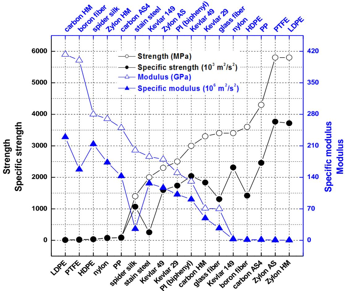
**Figure 1-16** Summary of mechanical properties of various materials. ( $\Delta$ ) and ( $\blacktriangle$ ) for the top X axis, and ( $\circ$ ) and ( $\bullet$ ) for the bottom X axis.
