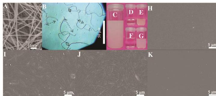
**Fig. 1.** SEM of short nylon-6 nanofibers (A); optical microscope photo of short nylon-6 nanofiber (B); digital photos of 0.1 wt% short nylon-6 nanofiber dispersion in DMF (C); pure TPU (D); nylon-6 short fiber/TPU dispersion (NT3.5) (E); PMMA solution in DMF (F); nylon-6 short fiber/PMMA dispersion (NP3.5) (G); SEM of surface morphologies of pure TPU film (H), NT2.5 (I), NT5.0 (J) and NP3.5 (K).
