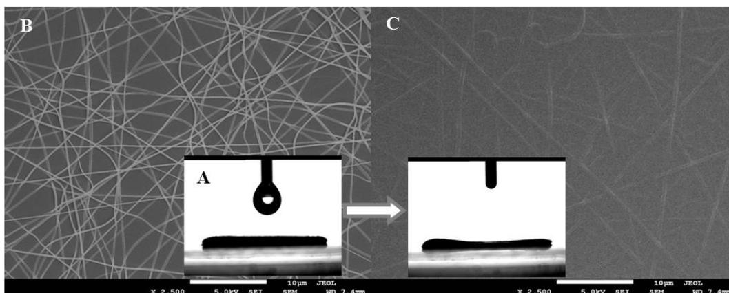
**Figure 2-6** DMF wetting behavior of nylon-6 nanofiber mat (A) and surface morphologies of 2-layered TPU/nylon-6 nanofiber composites (B: nylon-6 nanofibers on TPU film; C: nylon-6 nanofibers embedded in TPU resin). Scale bar = 10 µm.
