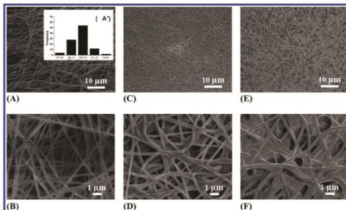
**Figure 3.** SEM images of (A) and (B) nylon-6 nanofibers, (C) and (D) MF/nylon-6 nanocomposite prepared by immersion into a MF solution of a concentration of 5 wt %, and (E) and (F) MF/nylon-6 nanocomposite made by immersion into a MF solution of a concentration of 15 wt %. (A') column diagram of the diameter distribution of nylon-6 nanofibers.
