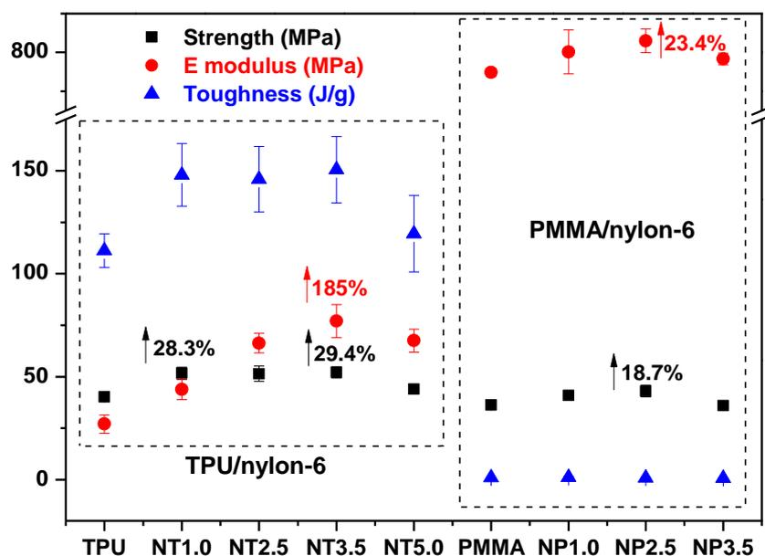
**Figure 2-11** Comparison of Strength (■), E modulus (●) and toughness (▲) of pure TPU film, PMMA film and short nylon-6 nanofiber reinforced composite films.
