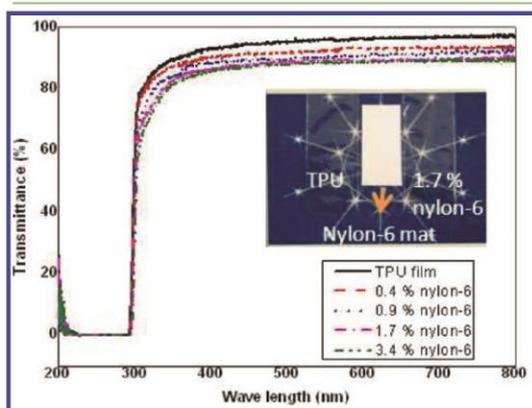
**Figure 8.** UV-vis spectra of TPU/nylon-6 nanofiber composite films (A) and digital photograph of transparent neat TPU film, nylon-6 nanofiber mat, and composite film (B).
