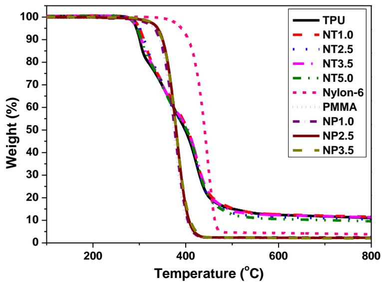
**Figure 5-S1** TGA curves of pure TPU film, pure PMMA film, nylon-6 nanofiber mat and short nylon-6 nanofiber reinforced composite films.
