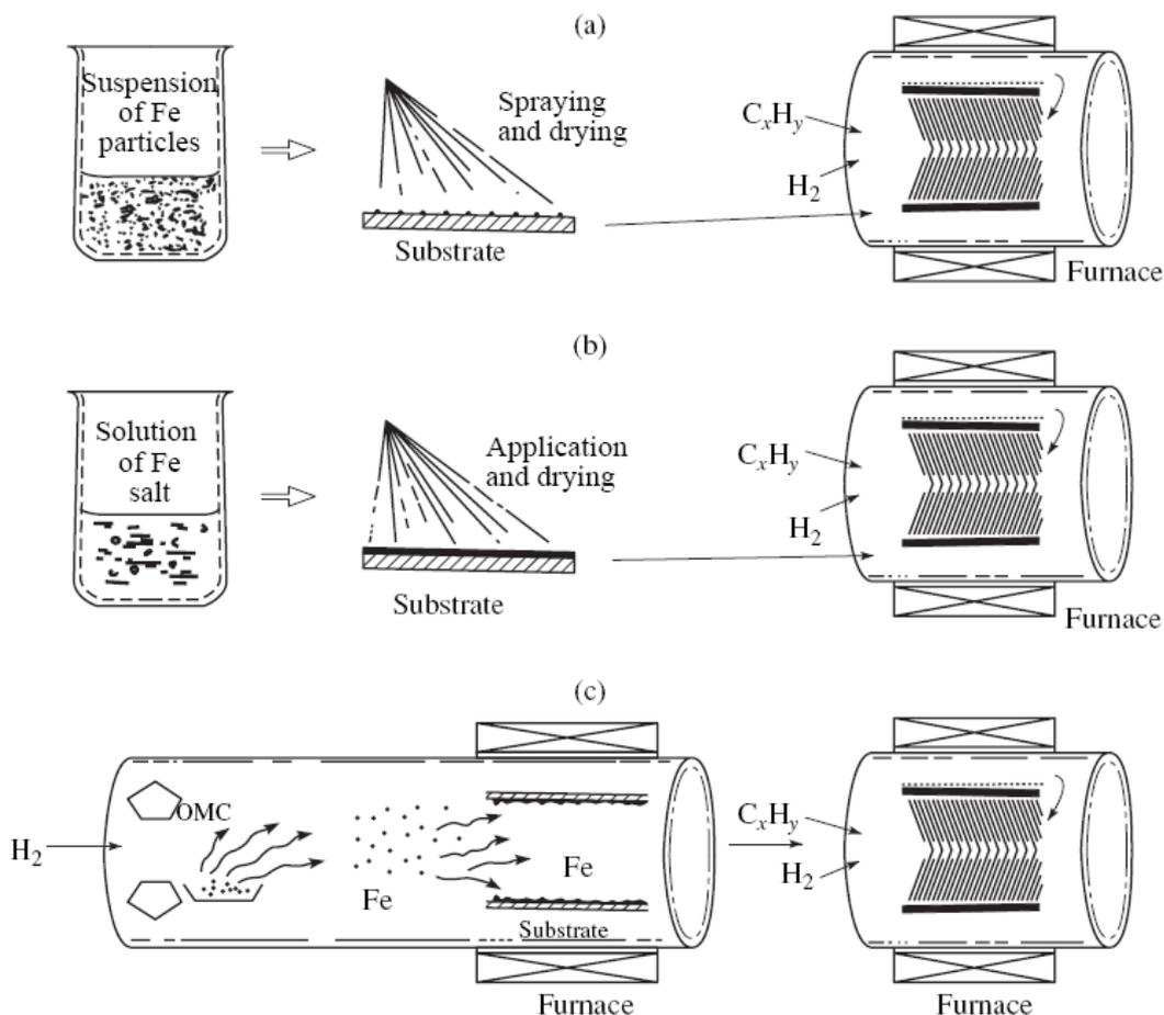
**Figure 1-8** Schemes of the growth of vapor grown carbon fibers on a substrate: (a) a catalyst is applied as a suspension of a fine iron powder in a solvent, (b) a catalyst is applied as a solution of iron compounds, and (c) iron-containing organometallic compounds (OMC) are introduced immediately into the reactor[81].
