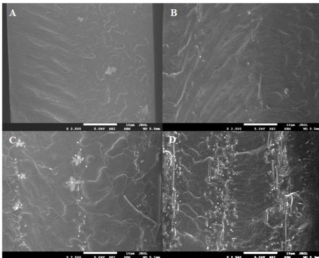
**Figure 2-8** Cross-section morphologies of neat TPU film (A) and laminated TPU/nylon-6 composites with 2 min (B), 4 min (C) and 8 min (D) electrospinning time on each layer. Scale bar = 10  $\mu\text{m}$ .
