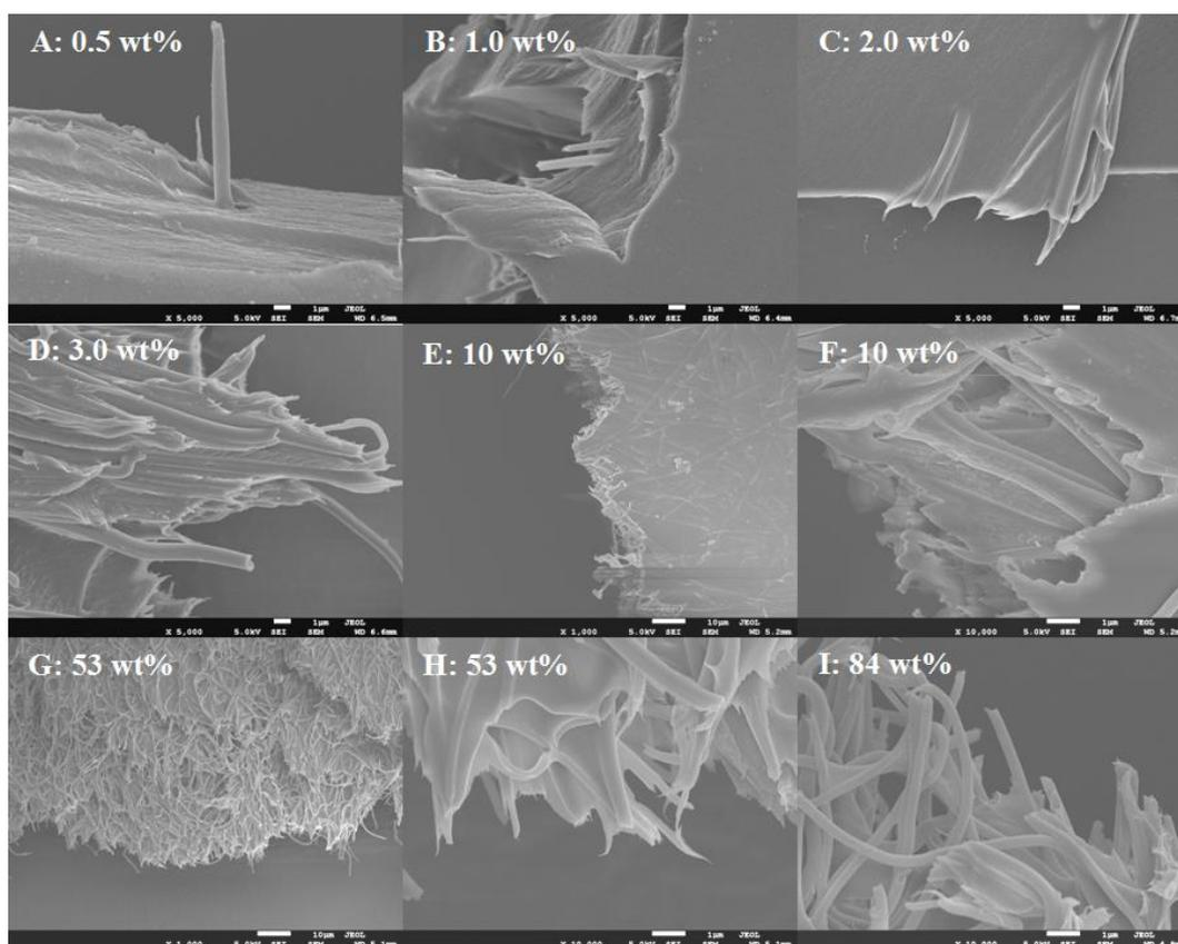
**Figure 2-16** Fractured surface morphologies of PIPICOF with different amount of short PI nanofibers (A, B, C, and D) and as-electrospun long PI nanofibers (E, F, G, H, and I). Scale bar of (A), (B), (C), (D), (F), (H) and (I) = 1  $\mu\text{m}$  and scale bar of (E) and (G) = 10  $\mu\text{m}$ .
