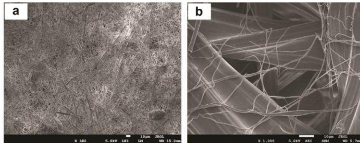
**Fig. 2.** SEM micrograph of dense layers of short electrospun PI nanofibers deposited from dispersion on filter paper (a) and at higher magnifications showing filter paper fibers with entangled nanofibers (b). Scale bar of (a) and (b) = 10 μm.
