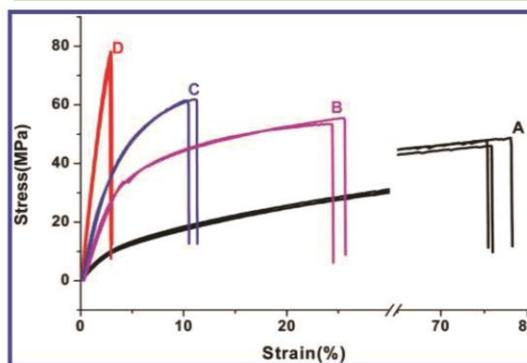
**Figure 6.** Typical stress–strain curves of MF/nylon-6 nanocomposites (method 1) with a content of nylon-6 in composites of (A) 100 wt %; (B) 62 wt %; (C) 30 wt %; (D) 13 wt %.
