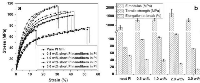
Fig. 3. Typical stress–strain curves of PIPICOF with different amounts of short PI nanofibers (a) and corresponding bar chart of mechanical properties (b).
