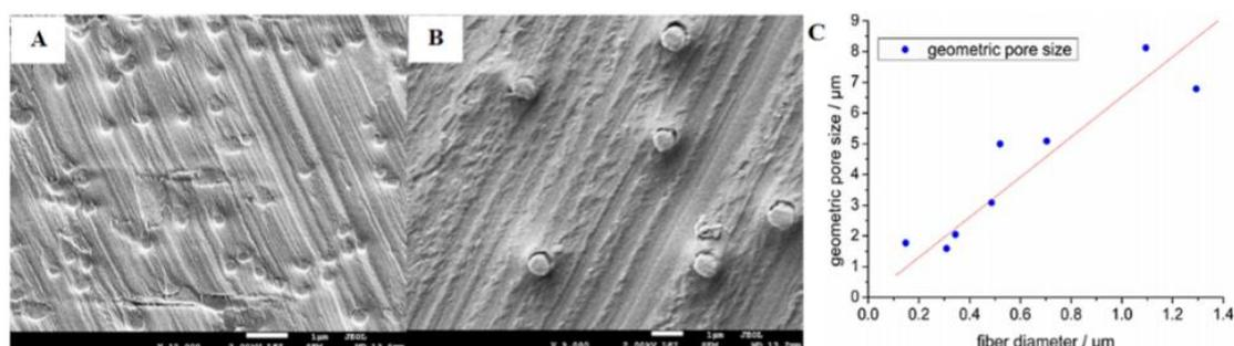
**Figure 1-3** Cross-section of PAN nonwovens embedded in an epoxy matrix with fiber diameter of A) 309 nm, B) 520 nm; and C) Dependence of geometric pore size on fiber diameters for PAN based nonwovens[126].
