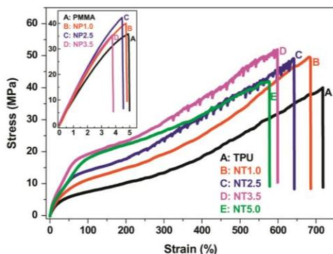
Fig. 3. Typical stress-strain curves of the pure TPU film, pure PMMA film and short nylon-6 nanofiber reinforced composites.
