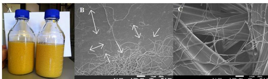
**Figure 2-14** Photograph of dispersions of electrospun fibers after cutting (A); SEM micrograph of short PI nanofibers (B) and SEM micrograph of short PI nanofibers deposited from dispersion on filter paper (C). Scale bar of (B) and (C) = 10  $\mu\text{m}$ .
