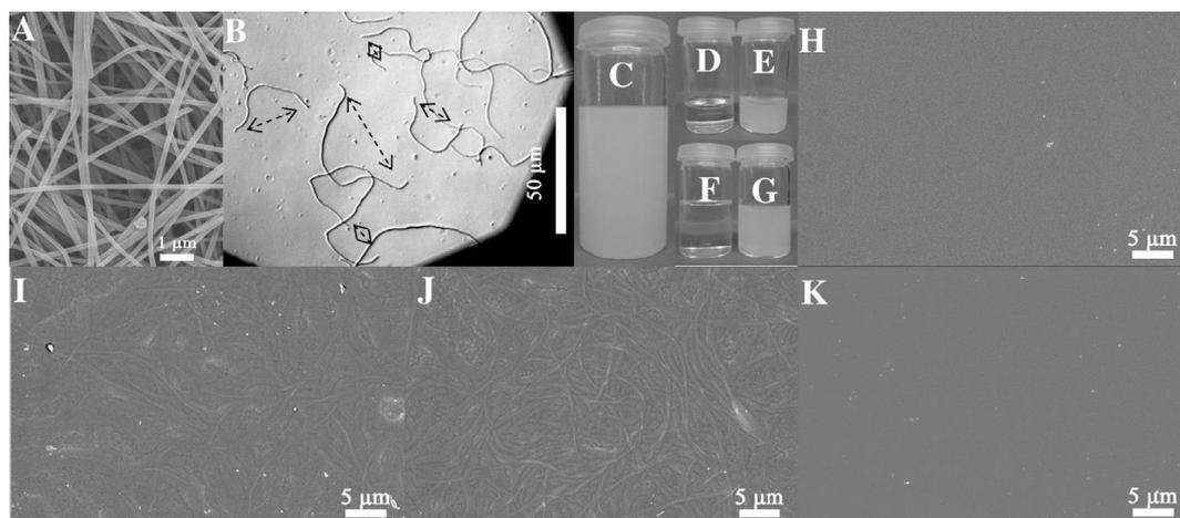
**Figure 2- 9** SEM of short nylon-6 nanofibers (A); optical microscope photo of short nylon-6 nanofiber (B); digital photos of 1.0 wt% short nylon-6 nanofiber dispersion in DMF (C); pure TPU (D); nylon-6 short fiber/TPU dispersion (NT3.5) (E); PMMA solution in DMF (F); nylon-6 short fiber/PMMA dispersion (NP3.5) (G); SEM of surface morphologies of pure TPU film (H), NT2.5 (I), NT5.0 (J) and NP3.5 (K).
