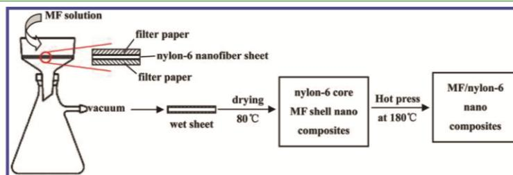
Figure 2. Schematic process for the preparation of the MF/nylon-6 nanocomposites by passing a MF solution through the nylon-6 nanomat and followed by hot-pressing (method 2).
