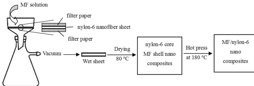
**Figure 2-2** Schematic process for the preparation of the MF/nylon-6 nanocomposites by passing MF solution through the nylon-6 nanomat and followed by hot-pressing (method 2).
