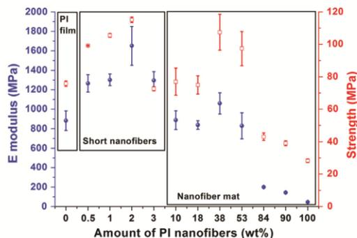
Fig. 5. Comparison of E modulus (●) and strength (□) of PIPICOF and PI self-reinforced nanofiber composites with as-electrospun PI nanofibers and a pure PI film.
