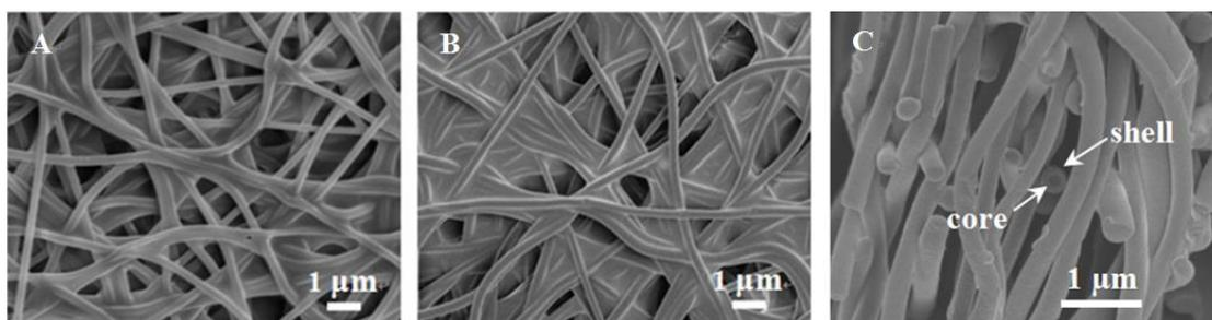
**Figure 2-3** SEM images of MF/nylon-6 nanocomposite prepared by method 1 with MF concentration of 5 wt % (A) and 15 wt % (B) and SEM image of MF/nylon-6 nanocomposite prepared by method 2 (C).
