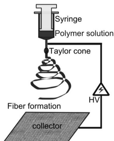
**Figure 1-12** Basic set-up for electrospinning.
