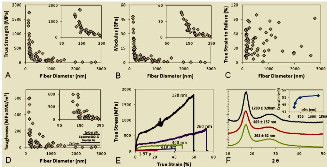
**Figure 1-6** Size effects in mechanical properties and structure of as-spun PAN nanofibers. (A) true strength; (B) modulus; (C) true strain to failure; (D) toughness (lines indicate comparison values for several high-performance fibers and spider silk); (E) typical stress/strain behavior; (F) XRD patterns for nanofiber bundles with different average fiber diameters and variation of degree of crystallinity with average fiber diameter (inset)[128].
