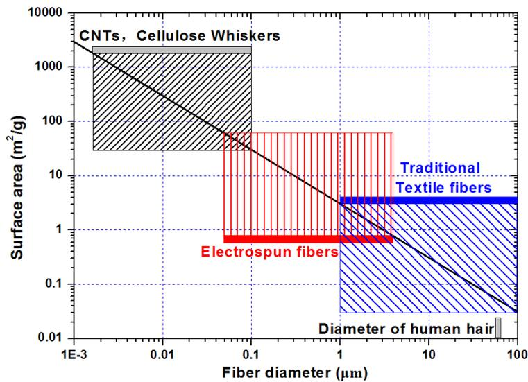
**Figure 1-4** Dependence of specific surface area on fiber diameter in nonwovens.
