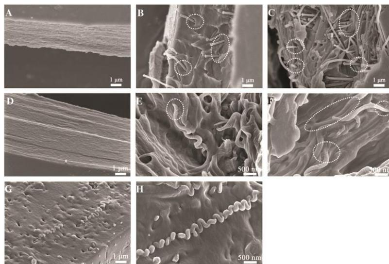
**Fig. 4.** SEM pictures of the tensile failure structure of pure PMMA film (A), NP2.5 (B), NP3.5 (C), TPU film (D), NT2.5 (E) and NT5.0 (F–H).
