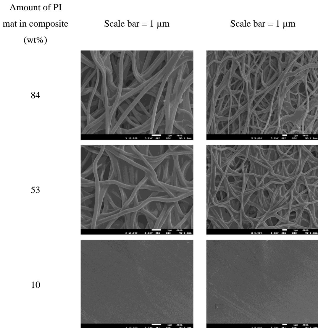
**Figure 6-S2** SEM photographs of the surfaces of PI self-reinforced composites using as-spun PI nanofibers.
