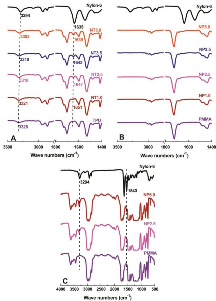
Fig. 2. (A and B) ATR-IR spectra of pure TPU film, pure PMMA film, nylon-6 nanofiber mat and short nylon-6 nanofiber reinforced TPU and PMMA composite films. (C) FT-IR spectra with transmission mode of pure PMMA film, nylon-6 nanofibers and composite films NP2.5 and NP5.0.
