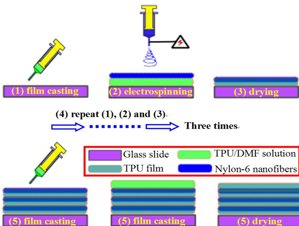
**Figure 2-5** Schematic of preparation of nylon-6 nanofiber reinforced TPU composite films.
