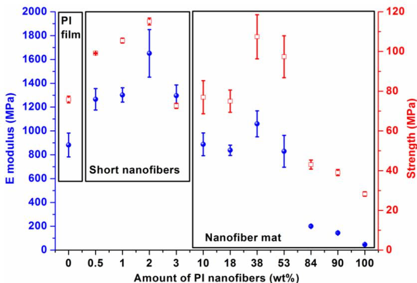
**Figure 2-15** Comparison of E modulus (●) and strength (□) of PIPICOF and PI self-reinforced nanofiber composite with as-electrospun PI nanofibers and a pure PI film.
