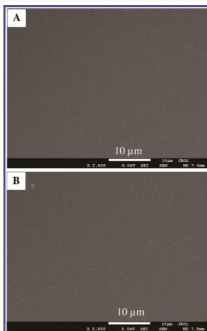
**Figure 4.** Surface morphologies of neat TPU film (A) and laminated TPU/nylon-6 nanofiber composite (B). Scale bar = 10  $\mu\text{m}$ .
