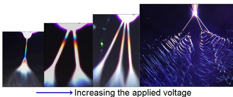
**Figure 1-13** Number of electrospinning jets as increasing the applied voltage[180].
