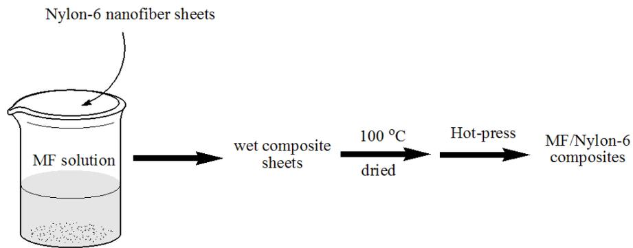
**Figure 2-1** Schematic process for the preparation of the MF/nylon-6 nanocomposites by immersing and hot-pressing (method 1).
