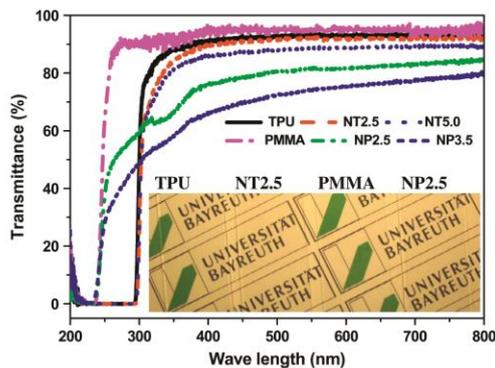
**Fig. 5.** UV–vis spectra of pure TPU film, pure PMMA film and short nylon-6 nanofiber reinforced composite films and digital photo of transparent neat films and composite films on glass slides.
