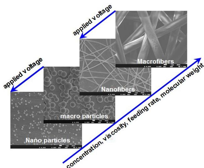
**Figure 1-14** The effect of some electrospinning parameters on the formation and the morphology of the particles and fibers.
