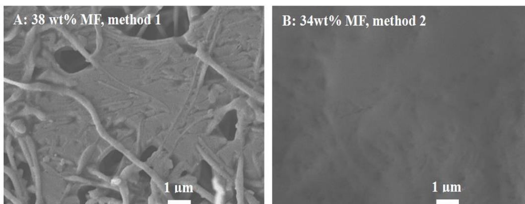
**Figure 2-4** Morphology comparison of the nylon-6/MF nanocomposites after hot-pressing.
