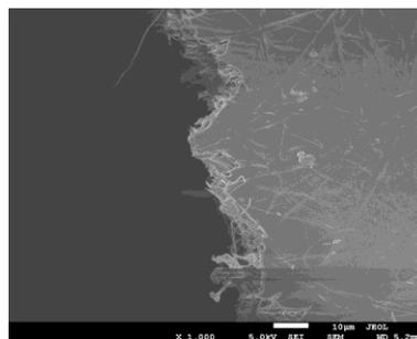
**Figure 6-S3** SEM micrographs of samples of PI self-reinforced PI nanofiber composites with different amounts of as-electrospun PI nanofibers after tensile tests.
