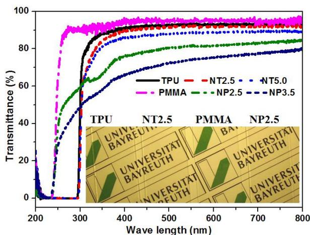
**Figure 2- 13** UV-vis spectra of pure TPU film, pure PMMA film and short nylon-6 nanofiber reinforced composite films and digital photo of transparent neat films and composite films on glass slides.
