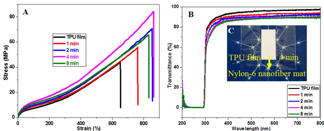
**Figure 2-7** Typical stress-strain curves (A), UV-Vis spectra(B) of TPU/nylon-6 nanofiber composites with different electrospinning time for each nanofiber layer and digital photograph (C) of nylon-6 nanofiber mat, transparent neat TPU film and composite film.
