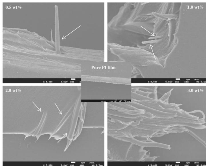
Fig. 4. Fractured surface morphologies of pure PI and PI/PI nanofiber-composite films with different amounts of short PI nanofibers. Scale bar = 1 μm.
