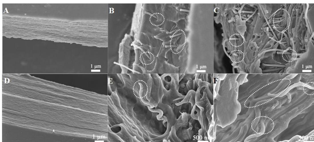
**Figure 2-12** SEM pictures of the tensile failure structure of pure PMMA film (A), NP2.5 (B), NP3.5 (C), TPU film (D), NT2.5 (E) and NT5.0 (F).
