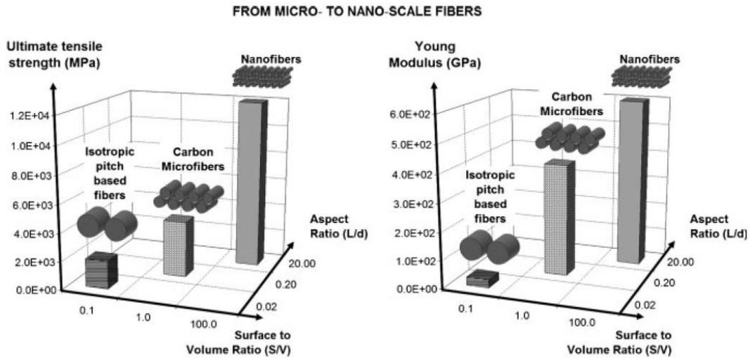
**Figure 1-5** From micro- to nano-scale fibers as reinforcement of bulk composites[125].
