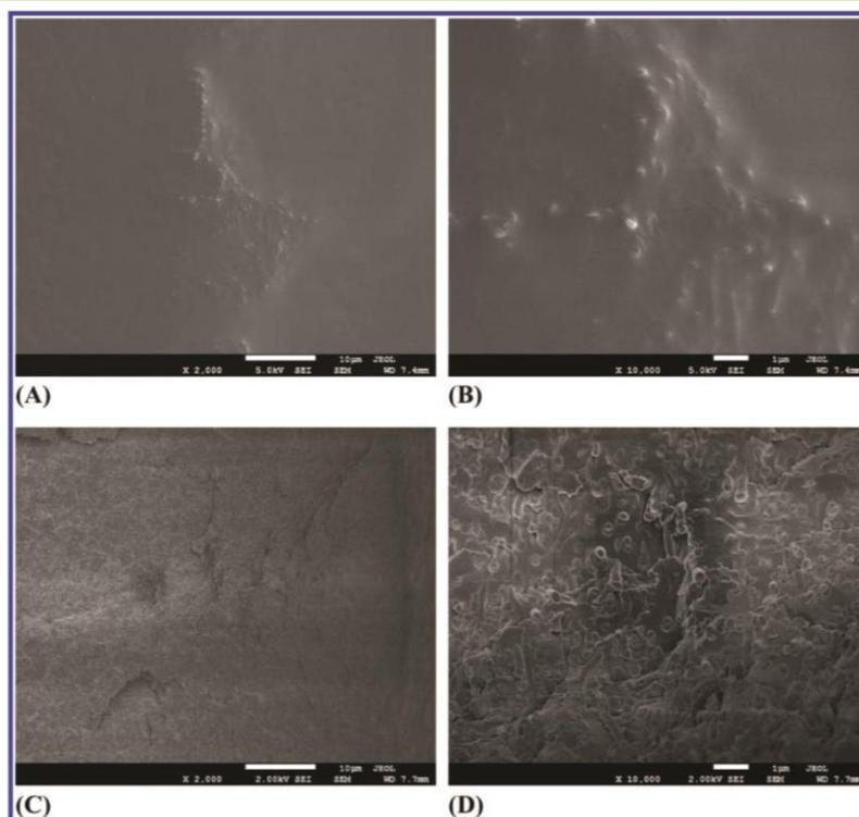
**Figure 7.** SEM images of fracture cross-section of composites (method 1) with a content of nylon-6 nanofibers of (A) and (B) 13 wt % and (C) and (D) 62 wt %. Scale bar: (A) and (C), 10  $\mu\text{m}$ ; (B) and (D), 1  $\mu\text{m}$ .
