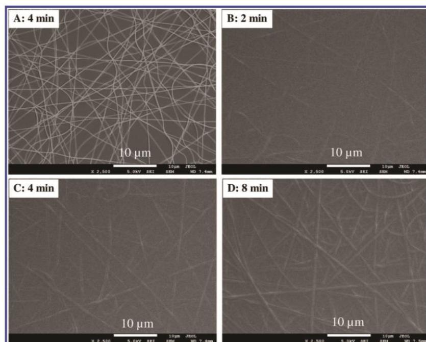
**Figure 3.** Surface morphologies of 2-layered TPU/nylon-6 nanofiber composite films (A: nylon-6 nanofibers on TPU film; B, C, and D: nylon-6 nanofibers embedded in TPU resin). The electrospinning time of A, B, C, and D were 4 min, 2 min, 4 min, and 8 min, respectively. Scale bar = 10  $\mu\text{m}$ .
