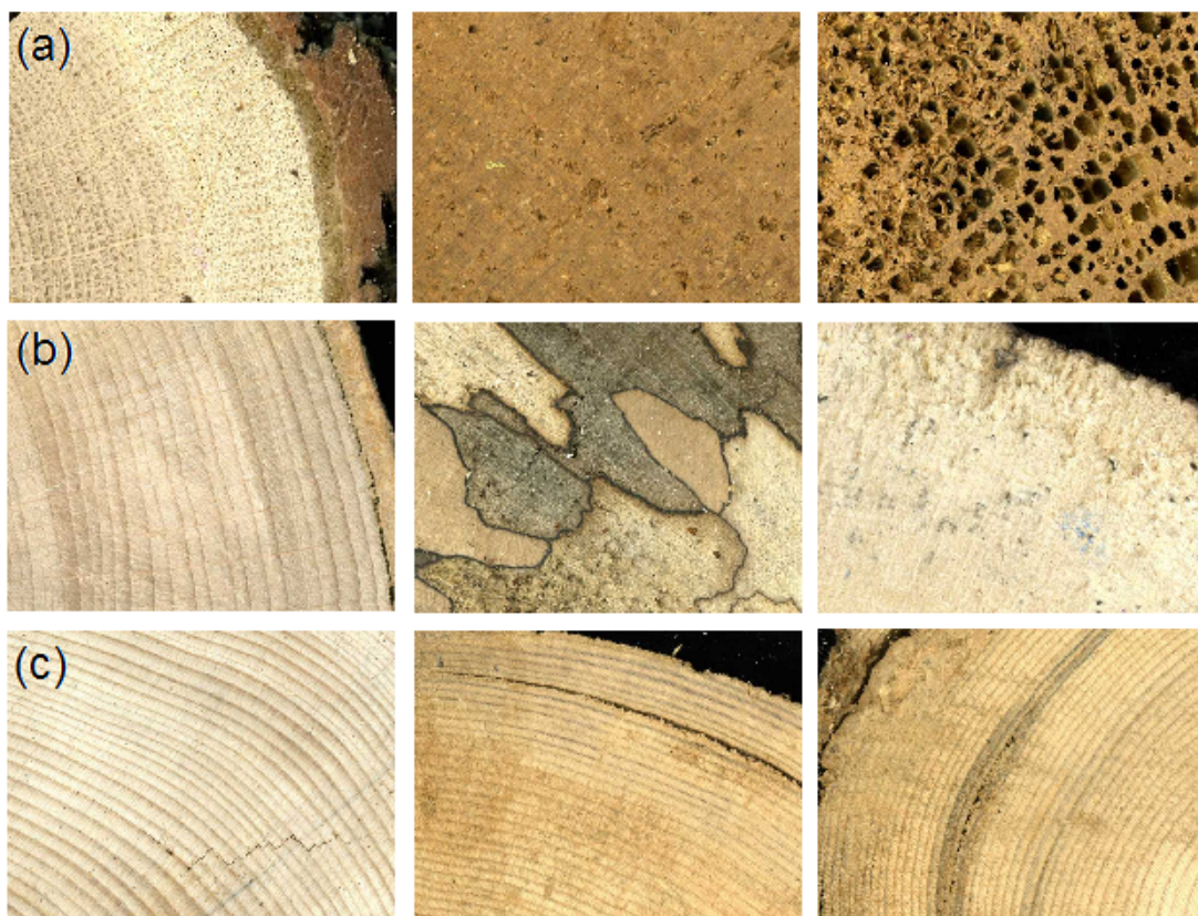
Fig. 2.2: Samples of coarse woody debris of Sessile oak (a), European beech (b) and Norway spruce (c) at different stages of decay.
